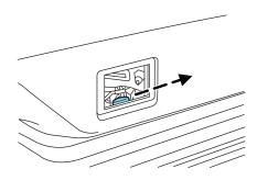
• For vehicles with power liftgate, pull the lock/unlock lever toward you (toward the front of the vehicle).
